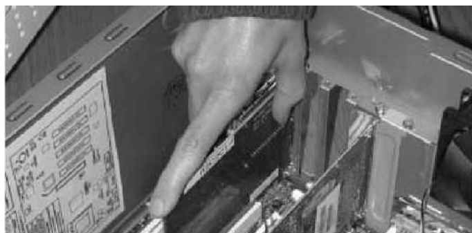
Figure 2.1: Inserting the DVB board into a PCI slot
